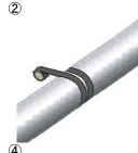
Measure the required length SC Flex, wrap symmetrically duct tape each one cycle to the axis of the cut.
