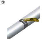
Along the center of a duct tape of the two, cut the inner layer material and glass wool and the outer layer material, with a sharp knife such as utility knife.
