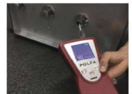
Factory exhaust air measurement
